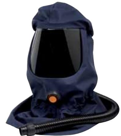
**Hood SR 561** A lightweight hood which protects the head and shoulders. Replaceable hood of Tyvek® with an easily adjustable head harness. Easily adjustable and comfortable neck seal of cotton. Visor of PETG. SR 561 is TH3 approved.
